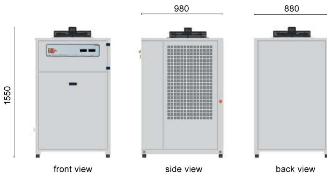
Fig. 7: Dimensions of external cooling system Tau 510 RSCi in [mm]
